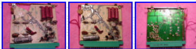
Attempting to rebuild the blown apart circuit board, PB-171A
